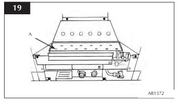
9.2 Place the rear panel against the rear of the box resting on the shelf. Then slide one of the side panels into the box
